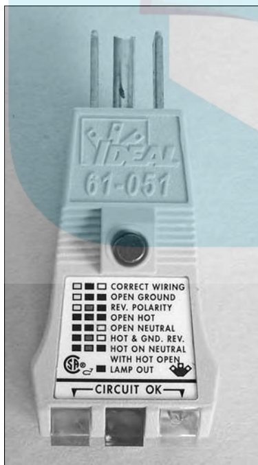
Figure 4-8: Receptacle and GFI tester close up.
